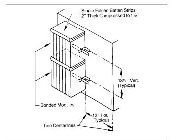
The Hefty Lock/Bonded 1100C module system is used in a wide range of applications in the temperature range up to 1100°C (2012°F). Typical applications include:
